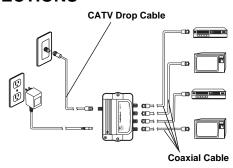
**Caution:** Use only coaxial cable (not supplied) to make the connections. Your local RadioShack store carries suitable cable.
